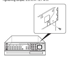
6 Use the four screws removed in step 1, to secure the DVR from the inside to the external disc unit.
